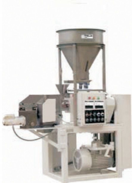
← MEFEDE-50 with 15 Kw Main Drive Motor (50 Kg/Hr. capacity)
