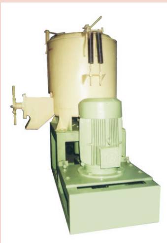
High speed Mixer for PVC Compounding 50 Kg batch cap.
