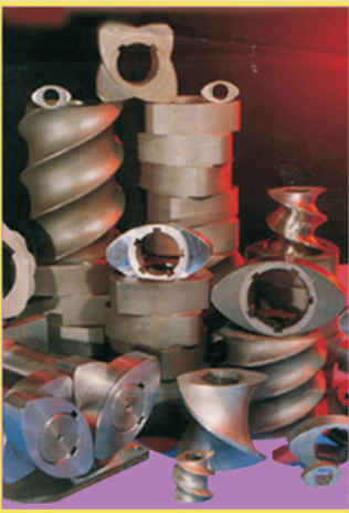
Screw elements for compounding TSE
